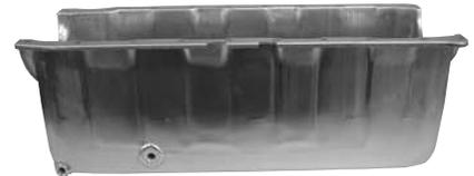
**Description:** The BBC pan is more for drag or marine use. It is made of 14 gauge steel to take the abuse of drag racing or marine use, it has 6 trapdoors, a back splash to keep oil from climbing up the back of the pan a louvered windage tray, crankscraper. It is available for both the GEN IV, GEN V & VI. also 7.5", 7.75", 8" Deep. Can also be used for agricultural use and Drag racing. Will clear 4.75 stroke.
