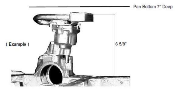
**Step 3:** Before final assembly, make sure all parts are thoroughly inspected and cleaned of any foreign debris, such as packing material, paper, stickers, etc. If the oil pan contains hinged trapdoor-style baffles, make sure they operate freely. It is advisable to reassemble the pan using Loc-tite on all nuts and bolts to help prevent them from loosening. Also, you should install the oil pan with the engine upright to ensure no trapdoors will be caught in an open position.
